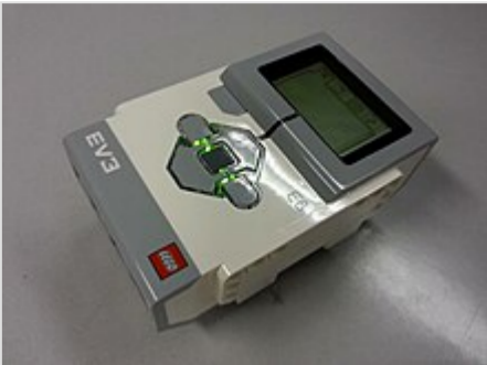
Lego Mindstorms EV3 brick has an ARM9 TI Sitara AM1x
