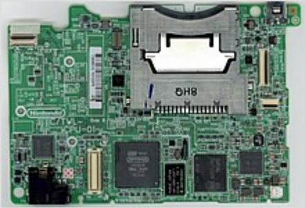
Nintendo DSi has a chip with an ARM9 and ARM7 core
