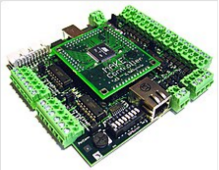
The Make Controller Kit with an Atmel AT91SAM7X256 (ARM) microcontroller
