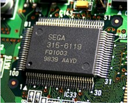
Yamaha AICA sound processor in Dreamcast game console [5][6][7]
