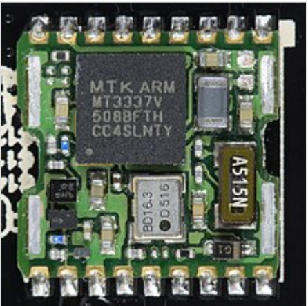
MediaTek MT3337V - ARM7EJ-S processor
