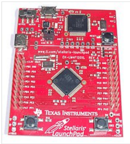
TI Stellaris Launchpad Board with LM4F120
